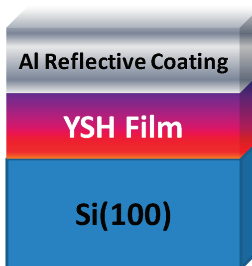
Figure 1. Schematic diagram of the layer sequence grown for thermal conductivity measurements. The Si substrate, YSH film, and Al top layer reflecting coating are as shown.
